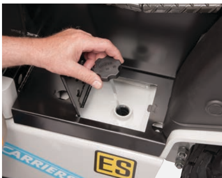
Access to hydraulic fluid located under door on right side step, for regular inspections and refills.
