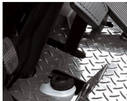
Two-piece diamond tread floorboard includes door to access brake fluid for visual level inspection and refills.
