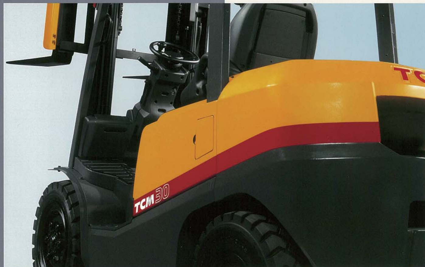
5% improved front and rear stability ratio (available for 2-3.5ton models) Stable and more consistent cargo handling as well as travel due to an improved stability ratio.
