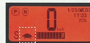
Speed limiter in operation
