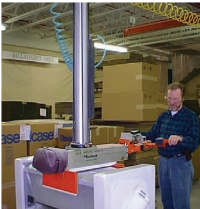
V-Lift mounted on a trolley/overhead bridge crane with an OD gripper end-effector handling furniture.
