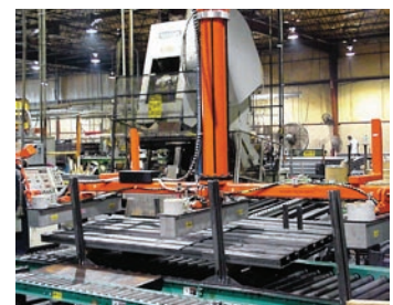
Magnet end-effector moving steel sheets in the assembly process.
