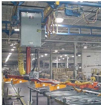
V-Lift mounted on a trolley/overhead bridge crane with a magnet end-effector for handling steel tubes.
