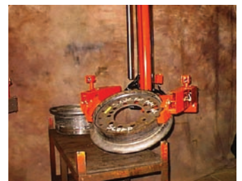
OD end-effector handling parts in an assembly process.
