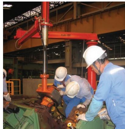
V-Lift mounted on a Positech Articulated Jib Boom with a custom end-effector handling rotary dies.
