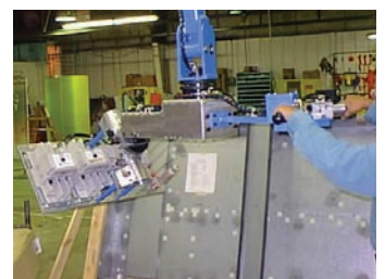
ID gripper end-effector handling electric panels.
