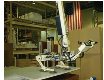
Vacuum end-effector handling parts in furniture assembly process.
