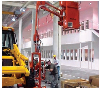
Overhead trolley mounted SAM and hydraulic powered end-effector installing tractor tires.
