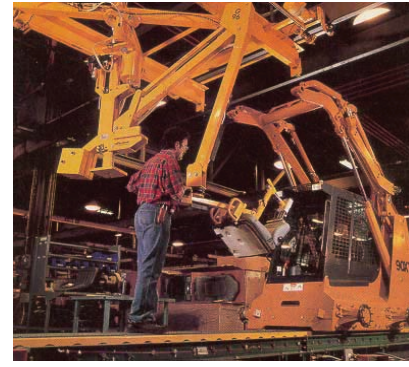
Overhead trolley mounted SAM and seat handling end-effector.
