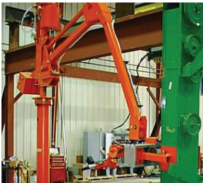
Pedestal mounted SAM used for lifting and positioning parts in assembly process of agricultural equipment.
