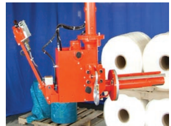
Expanding mandrel end-effector handling rolls of paper.
