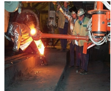
OD gripper end-effector used in foundry to handle SEN.
