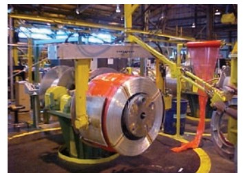
OD grip end-effector picks, rotates and unloads coil.
