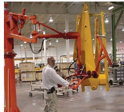
Pedestal mounted TPA loading and unloading backhoe parts on paint-line.
