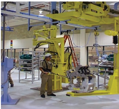
Pedestal mounted TPA loading engine blocks.
