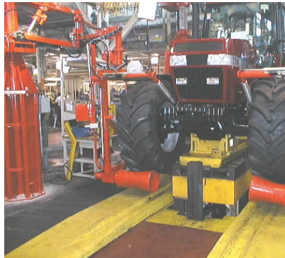
Pedestal mounted TPA installing 1,000 lbs. tires on a tractor.
