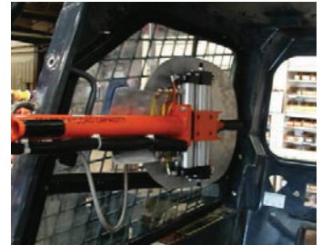
Vacuum end-effector rotates, flips, and installs left and right hand windows in cab assembly.
