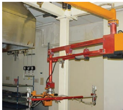
Optional 360° middle joint allows the LodeArm to maneuver in tight work cells, while handling silicon rods.
