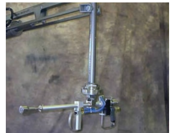
Mechanical end-effector is designed to hold a high pressure wand to minimize operator fatigue.
