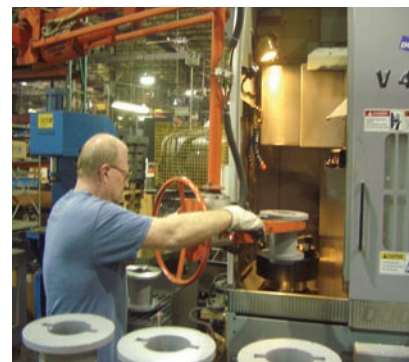
Pedestal mounted LodeArm loading and unloading castings from a machining center.
