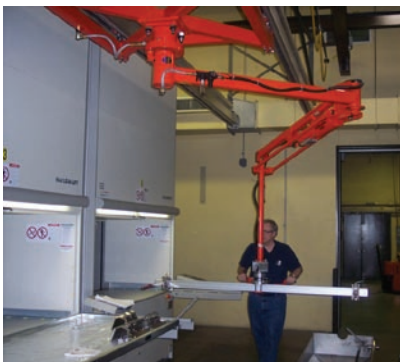
Trolley mounted LodeArm with fork end-effector loading and unloading trays from an AS/RS.
