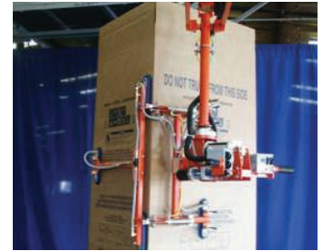
Vacuum end-effector picks box from horizontal, pitches to vertical, unfolds and positions over appliance.
