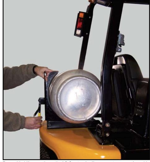
For multi-shift operations, the LP Gas truck offers non-stop operation with only the need to change LP Gas tanks between shifts. This truck eliminates the need for costly battery charging systems and the related hazards.
