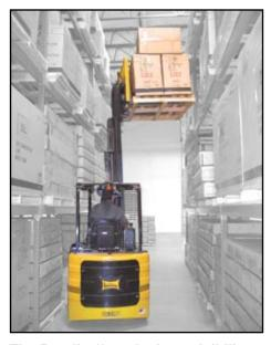
The Bendi offers the best visibility while stacking. The entire length of the load is visible to the operator during stacking. There is no rear end swing during stacking, so product and rack damage is eliminated.
