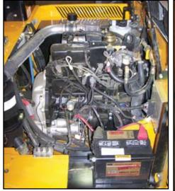
The LP Gas Bendi is easily serviced by opening side doors. All the major maintenance items are accessible including: oil and fuel filters, distributor, spark plugs, and fuel systems.
