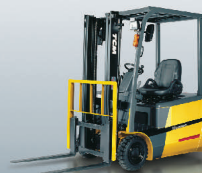
FTB18-7 Max. Capacity: 1,750kg (3,500lb) Load Center: 500mm (24 in.)
