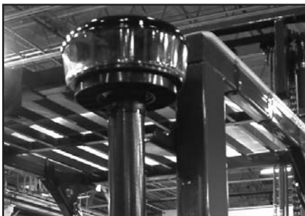
Air intake pre-cleaner for extended filter life.
