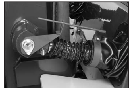
Tilt cylinder boots or tilt cylinder covers for protection against dirt and dust. Mast tilt gauge provides visual indication for vertical alignment of mast.
