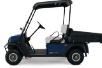
HAULER 800 13.5-hp Gas Engine or 48-Volt Drivetrain Load Capacity: 800-lb. (360 kg)
